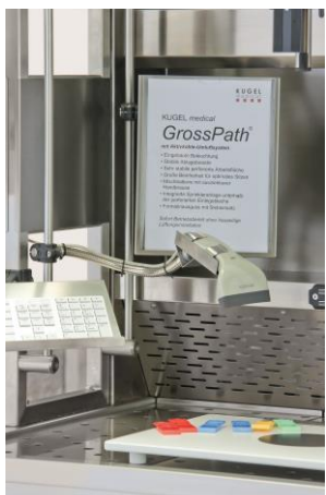
Swivelling scanner holder laterally mounted to the side rails FH-SCAN-SS-300 Art. No. 060.100.105
