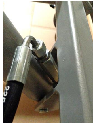
Brake valve installed at at a HTW
