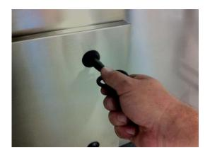
Open the inspection hole using the square key and remove the cover completely.
