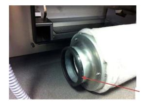
The sealing ring of the cartridge is to be checked upon good condition **before** inserting the filter cartridge!
