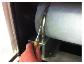
Open both connecting clips using a wrench and remove the filter cartridge.
